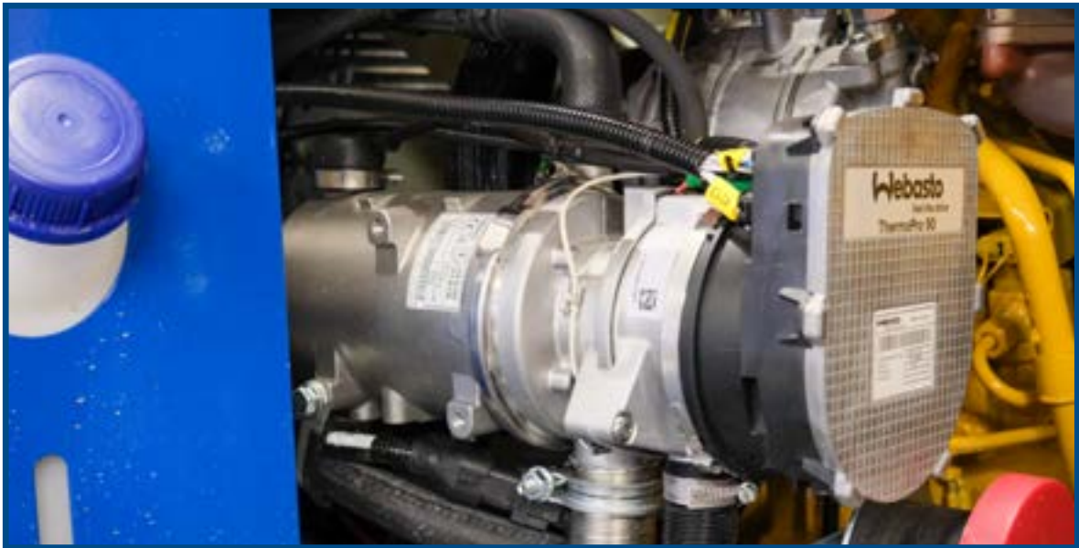
Webasto Thermo Pro 90, heats the engine and cab. Can be started with timer function, remote start from Rottne Connect, or via button in the cab.
